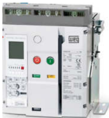
Figura 22 Disjuntor aberto ABWC1600, In 800~1.600 A, Icu = 50 kA @ 380 V, Ics = 100% Icu
