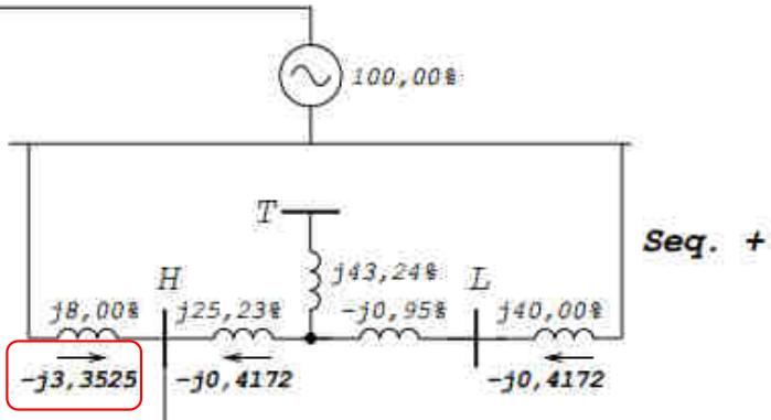
$$\hat{i}_{A_{138}} = 3,3525 \angle -90^\circ + 3,3525 \angle -90^\circ + 2,8978 \angle -90^\circ$$
