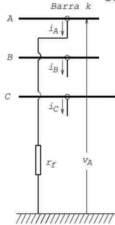
$$i_B = i_C = 0 \quad v_A = i_A r_f \quad \begin{bmatrix} \hat{v}_{A+} \\ \hat{v}_{A-} \\ \hat{v}_{A0} \end{bmatrix} = \begin{bmatrix} \hat{e}_A \\ 0 \\ 0 \end{bmatrix} - \begin{bmatrix} Z_{k,k}^+ & 0 & 0 \\ 0 & Z_{k,k}^- & 0 \\ 0 & 0 & Z_{k,k}^o \end{bmatrix} \cdot \begin{bmatrix} \frac{\hat{i}_A}{3} \\ \frac{\hat{i}_A}{3} \\ \frac{\hat{i}_A}{3} \end{bmatrix}$$
