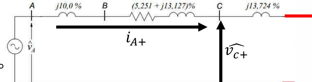
$$\widehat{v}_{c-} = 0 - 23,716\angle 77,21^\circ \times 1,1357\angle -83,15^\circ$$
