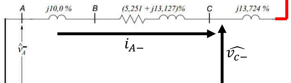
$$\widehat{v}_{c-} = 0,269\angle 174,06^\circ pu$$
