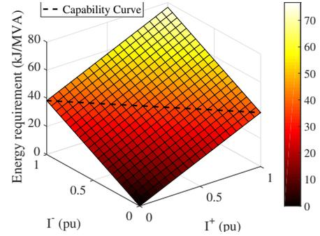
Fig. 3. Storage energy requirement for MMC considering negative sequence injection.
