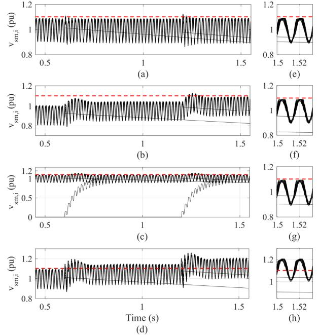
Fig. 4. Effect of the redundancy strategies in the dynamic of the SM voltages of the MMC: (a) RAS; (b) RASO; (c) RSS; (d) SR; (e) Detail for RAS strategy; (f) Detail for RASO strategy; (g) Detail for RSS strategy; (h) Detail for SR strategy.
