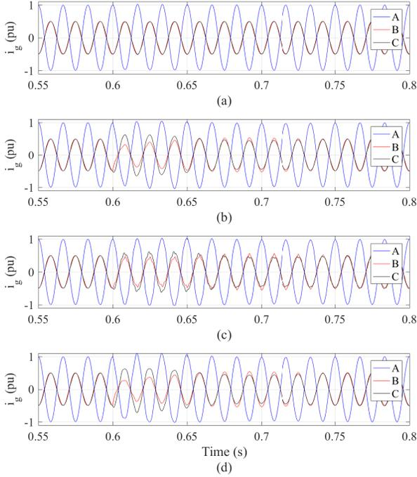
Fig. 5. Effect of the redundancy strategies in the grid current dynamic behavior: (a) RAS; (b) RASO; (c) RSS; (d) SR.
