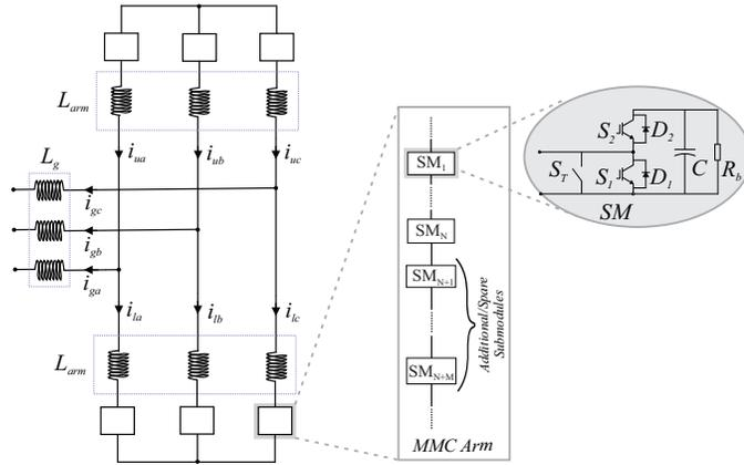
Fig. 1. Schematic of the DSCC-MMC STATCOM.
