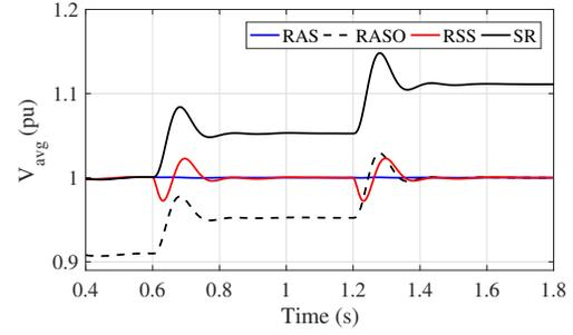
Fig. 6. Effect of the redundancy strategies in the SMs average voltage dynamic behavior: (a) RAS; (b) RASO; (c) RSS; (d) SR.
