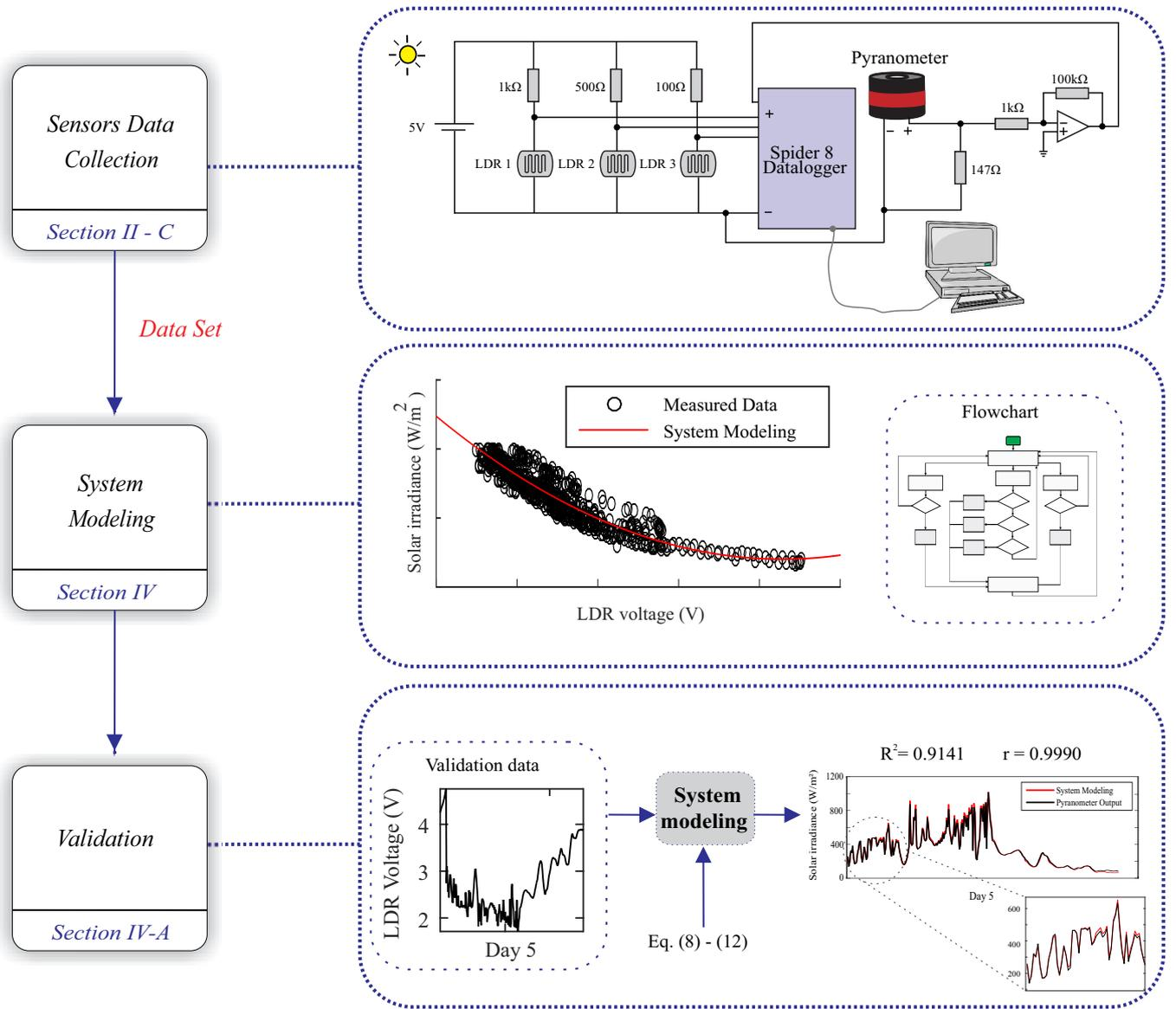
Fig. 3. Electrical schematic of the connections for data collection with pyranometer and LDRs.
