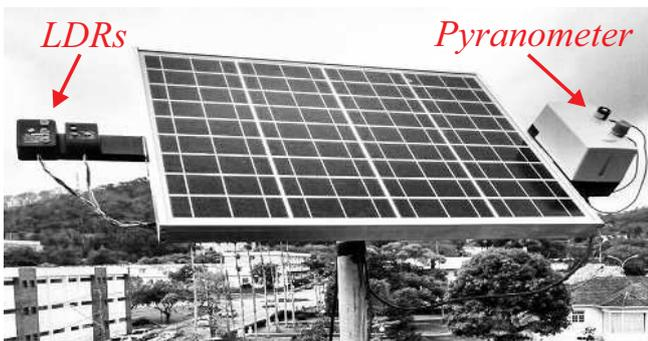
Fig. 4. Platform for data collection of LDRs and pyranometer sensors.
