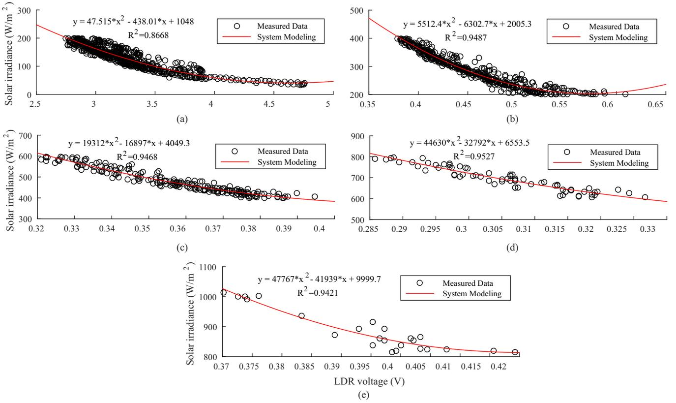
Fig. 8. Polynomial regression for Cases (a) I, (b) II, (c) III, (d) IV and (e) V, selected according to the coefficient of determination.
