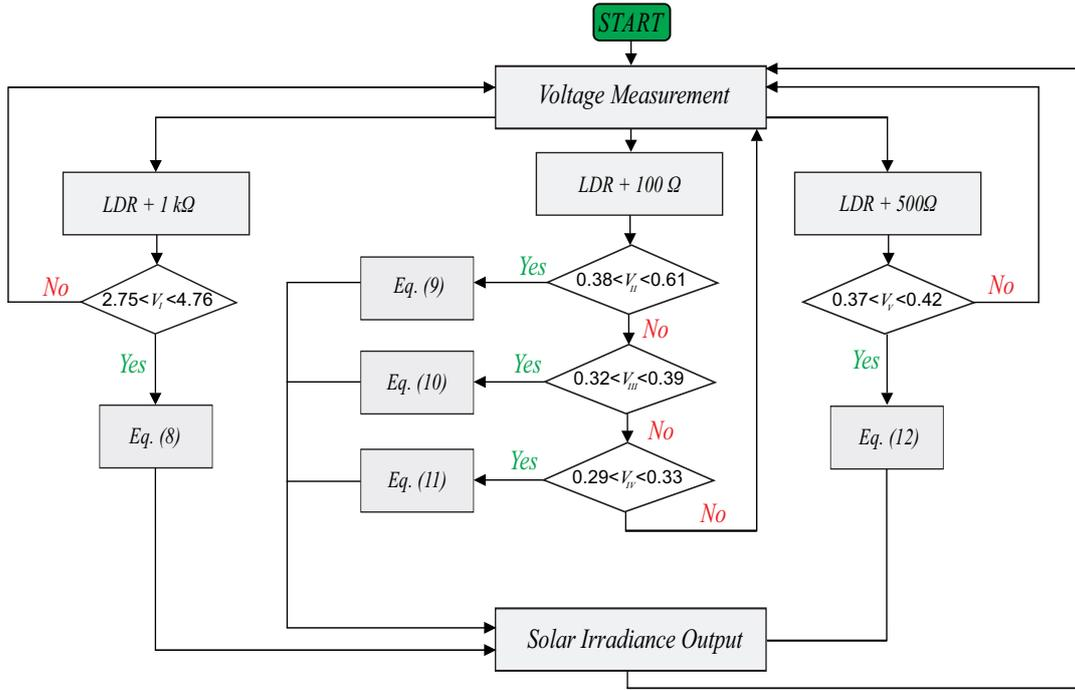
Fig. 7. Algorithm flowchart implemented to read LDR voltage and return the corresponding solar irradiance.
