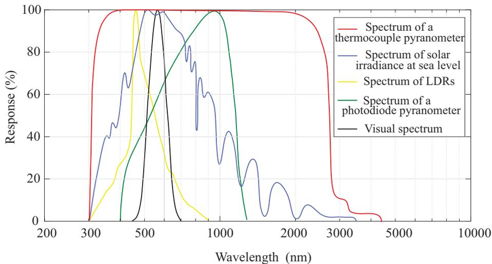
Fig. 2. Irradiance spectrum response of the sensors: photodiode pyranometer, thermocouple pyranometer and LDR; and of the solar irradiance at sea level. Adapted from [10].
