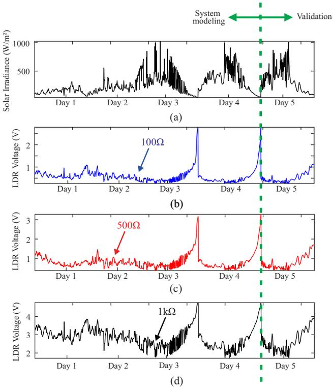
Fig. 5. (a) Solar irradiance 5-days profile. LDR voltage 5-days profile connected to the: (b) 100  $\Omega$  resistor. (c) 500  $\Omega$  resistor. (d) 1 k $\Omega$  resistor.
