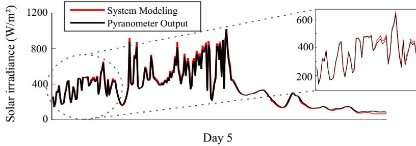
Fig. 9. Irradiance output read by the LDR after compiling the flowchart Fig. 7, compared to the reference for the validation data.
