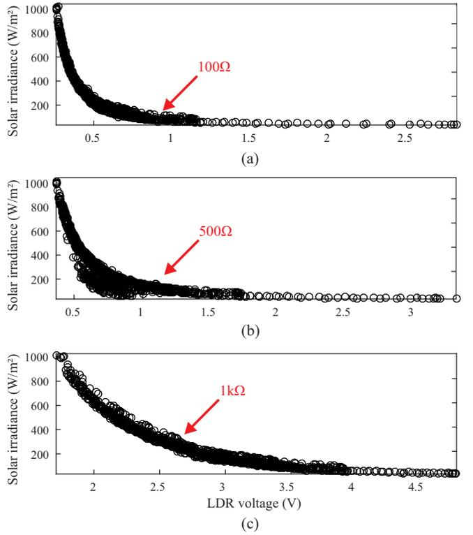
Fig. 6. Solar irradiance  $\times$  LDR voltage connected to the (a) 100  $\Omega$  resistor. (b) 500  $\Omega$  resistor. (c) 1 k $\Omega$  resistor.
